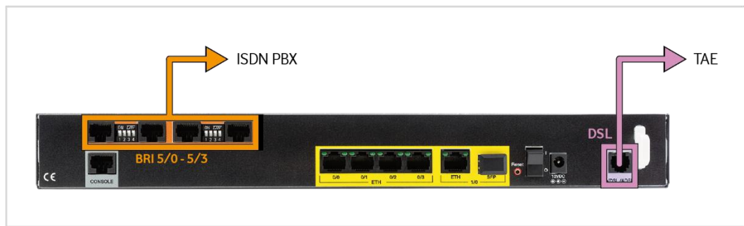
Fig. 4: Anlagen-Anschluss Plus, Connecting hardware with PlusBox 341, ISDN Voice only – Detail
