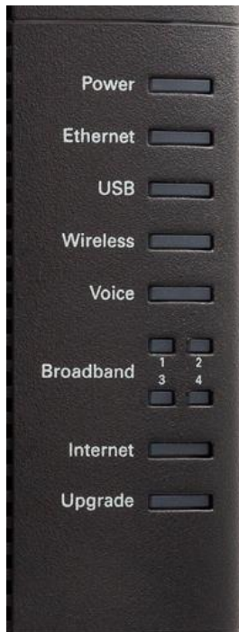
Abb. 11: Frontseitige LED am SDSL-Modem Technicolor TG670s (Acht draht)
