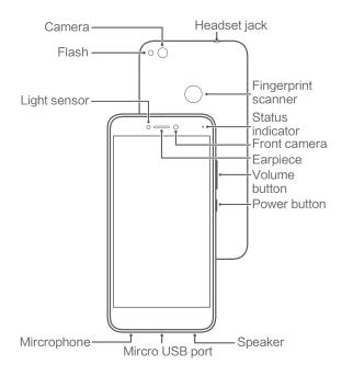
On not cover the light sensor, as this may affect some of the phone's functions. When using a screen protector, ensure that it has a purpose-built cutout for the light sensor.
