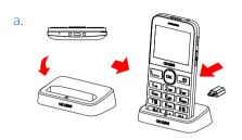
To charge the phone, you can place the cradle charging connector of the phone to the cradle, then connect battery charger to the cradle and plug into the socket.
