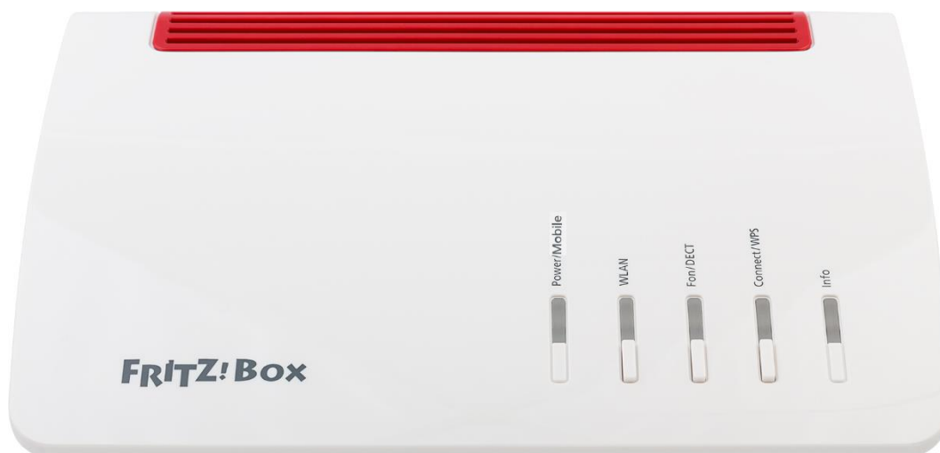
Abb. 18: LED an der FRITZ!Box 6850 (Indoor)
